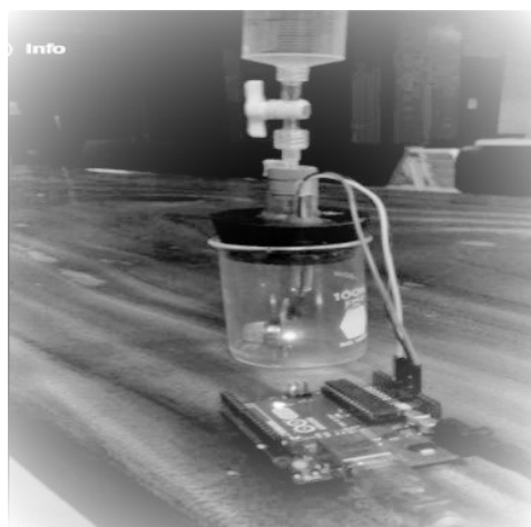
Figure 1 Gas sensing set-up showing airtight gas chamber (middle), Arduino microcontroller board (foreground), and syringe pump with valve (top).
